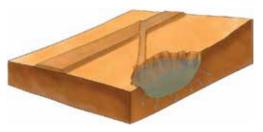
Figure 3 Rolling dip evacuating runoff generated by road to nearby pond *Credit*: illustration by Jochem van der Zaag (www.metameta.nl)
