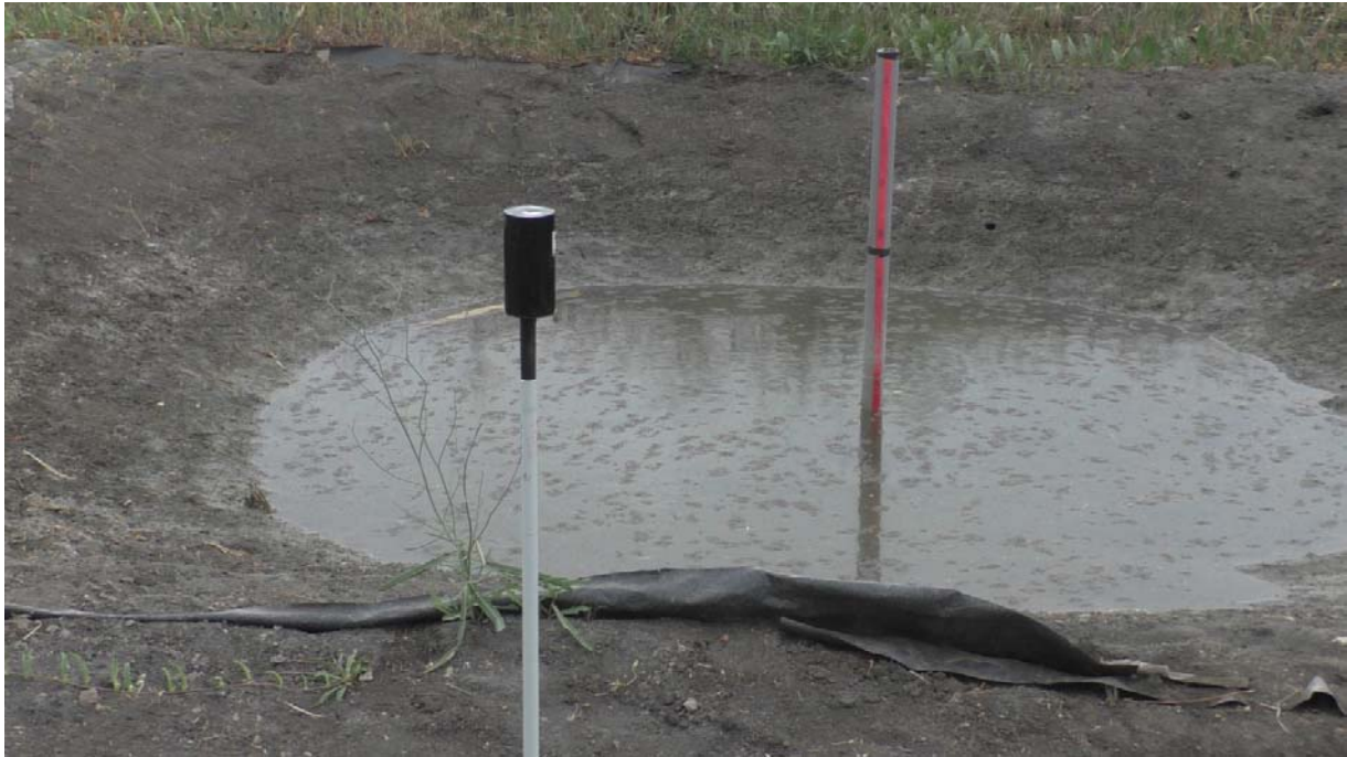
Figure 7: A pipe with a tape attached on the outside to help monitor water level.
