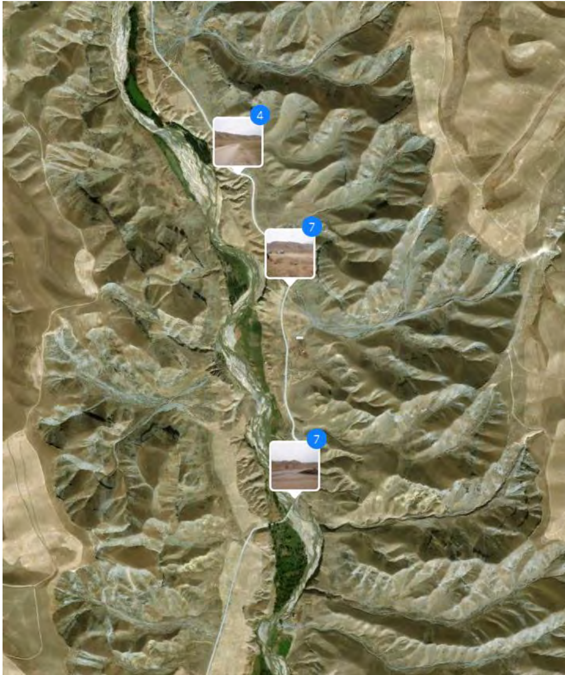
Map 3: the canyon along which the irrigation dam was planned (North side). The map shows the secondary erosion channels that contribute to siltation and building up high water levels in the Isfara River.
