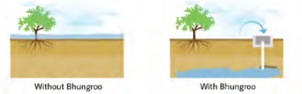
Plate 24: Tube recharge well collecting excess water for recharge (Source: Momentum4Change.org)
