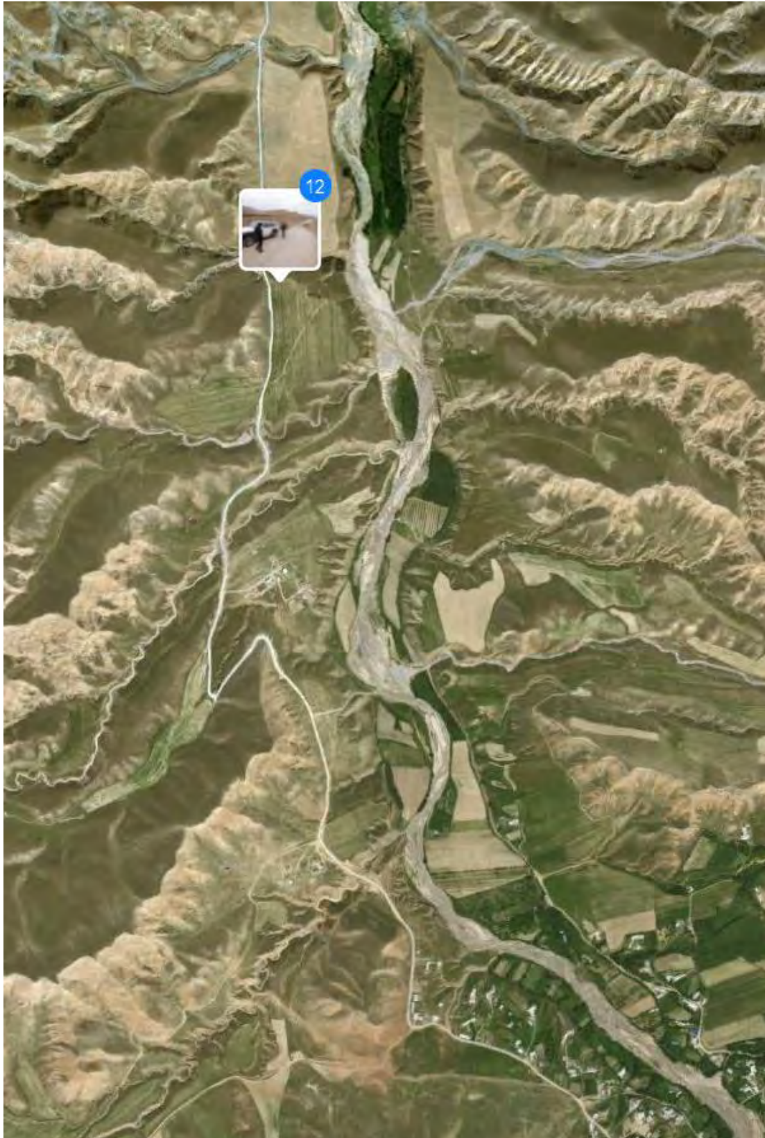
Map 4. The map shows the five erosion gullies where the road intersects seasonal streams, while the slopes above are severely eroded
