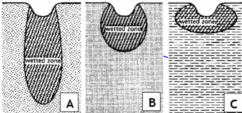
Figure 6 wetting patterns in soil, A-sand, B-loam, C-clay (source: FAO)
