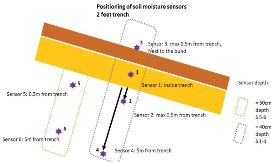
Figure 7 overview of positioning of soil moisture sensors
