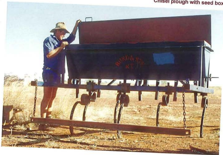
Plate 54. Chisel plough with seed box.
