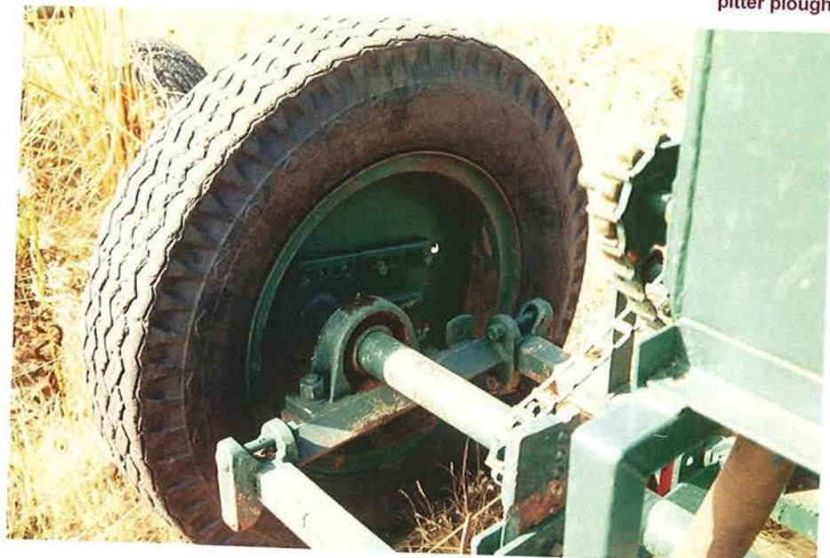
Plate 58. Eccentric axle on pitter plough.
