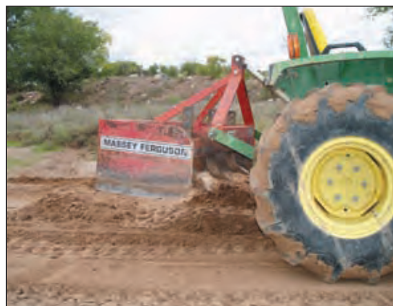
Photo IX-5: Farm tractor with a box scraper and rippers.
