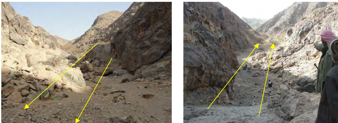
Figure #Potential location of small rural feeder road crossing small wadi stream and the road body may act as recharge/storage dam
