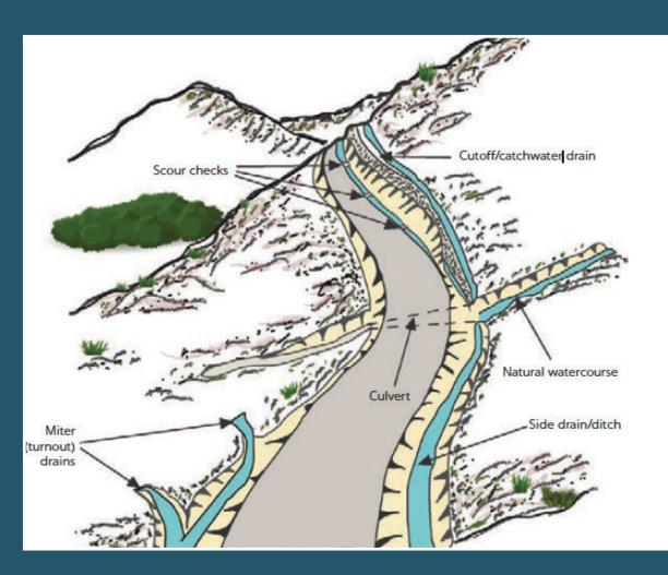
Well-developed drainage system collecting water and making it possible to route to areas of beneficial use
