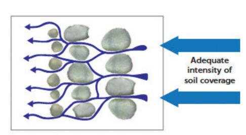
Use rocks (where available) or grasses on the road sides to dissipate water running from the unpaved road surface and avoid erosion
