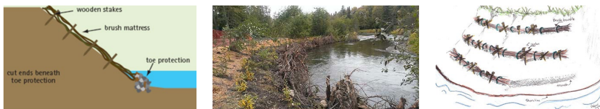
Figure 21 Impression from possible nature-based solutions: From left to right: brushwood mattresses with toe protection, root wads, fascine bundles. More illustrations, pictures, and notes on their applicability for different zones of Bangladesh will be provided in the forthcoming guidance note.
