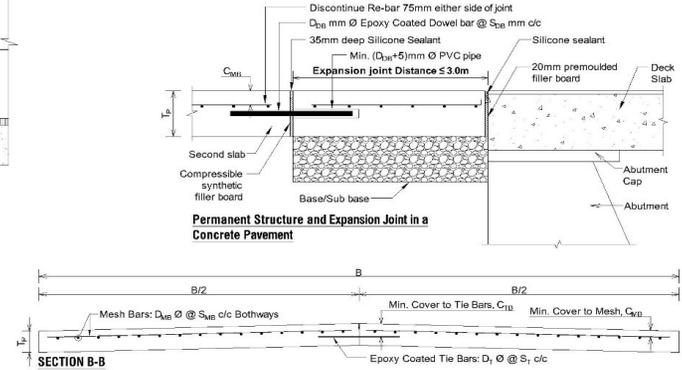
**Permanent Structure and Expansion Joint in a Concrete Pavement**
