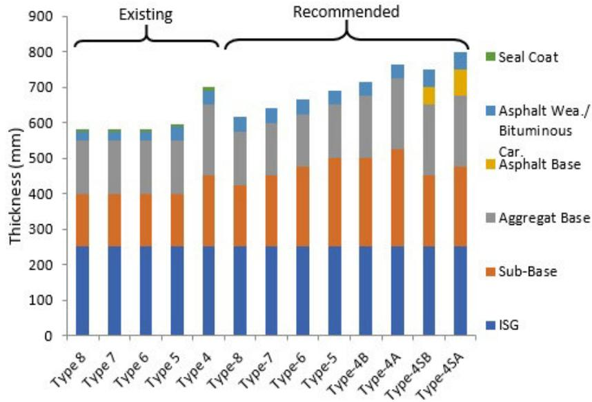
Figure 1: Comparison of Pavement Thickness
