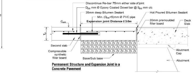
**Permanent Structure and Expansion Joint in a Concrete Pavement**
