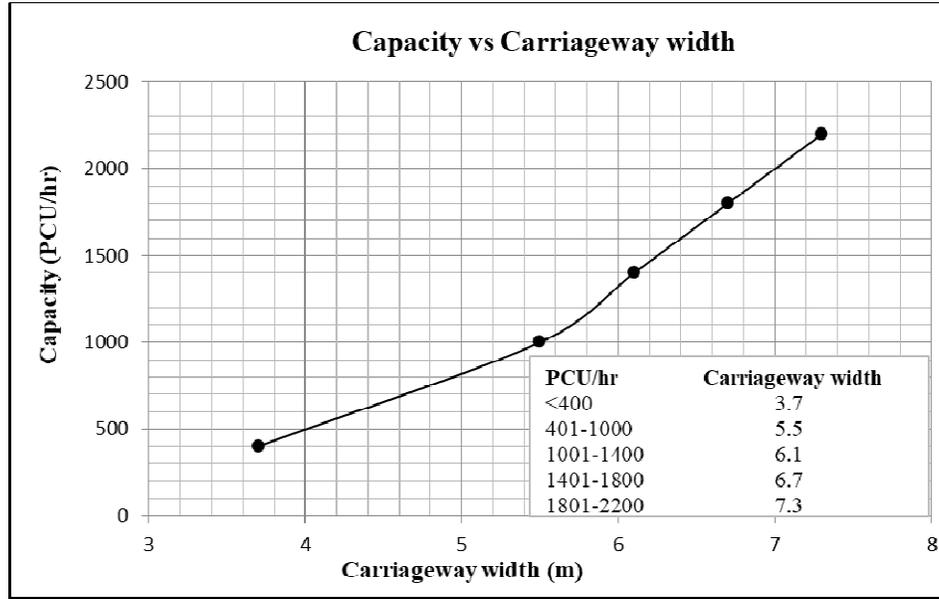
Figure 2: Relationship between Roadway Capacity and Carriageway Width
