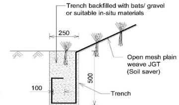
**Detail "Y" : Bottom Trench Cutting for JGT anchorage**
