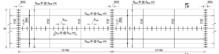
**REINFORCEMENT DETAILS OF RIGID PAVEMENT**
